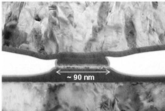
Fig. 10. TEM image of a typical TuMR reader device as seen by the recording disc.
