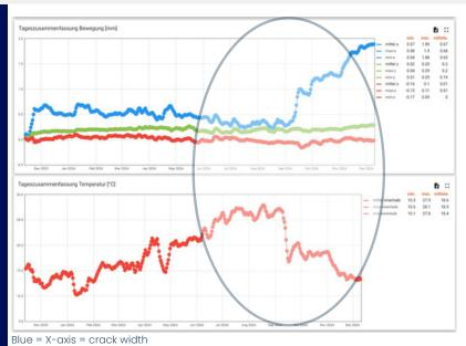
In September 2024, an increase of 1.2 mm in the X-axis can be observed. Temperature indexed due to a simultaneous drop in temperature clearly visible.
